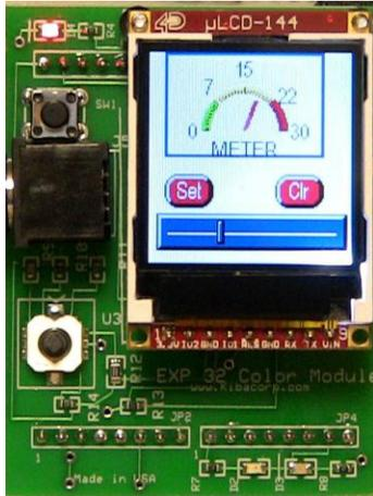
Here's a color carrier and uLCD-144 module shown running meter demo.
