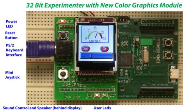
Figure 1 Color Carrier Module in operation with ULCD-144 and 32 bit Experimenter
